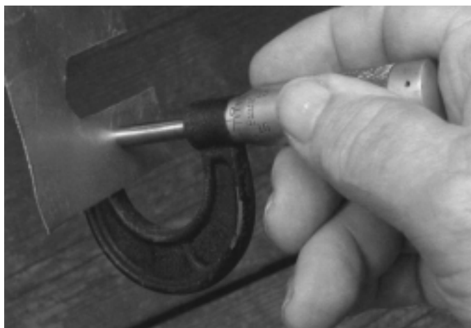
Figure 9-66. Measuring shim stock with micrometer
